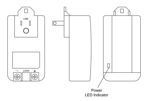
Description: Plug-in Class II Regulated Power Supply with LED power indicator.
